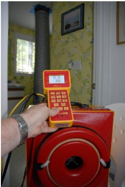
The same process can be used to test bathroom fans. The duct tester can be connected a box that covers the fan or grille. Because of the powered flow into the fan being tested, the measuring device (duct tester) is essentially invisible to the fan being tested, offering no resistance or impediment to the flow.
